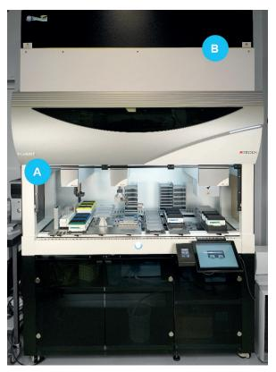
Figure 1: A Fluent Automation Workstation (A) fitted with a vertical laminar flow HEPA hood (B) used for the cell seeding and medium exchanges.
