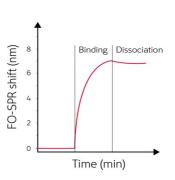
**3.** Spectrometer readout is converted to real-time binding and dissociation curves.
