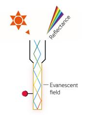
**2.** Mass difference changes refractive index, altering the spectrum of reflected light.
