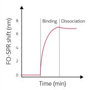
**3.** Spectrometer readout is converted to real-time binding and dissociation curves.
