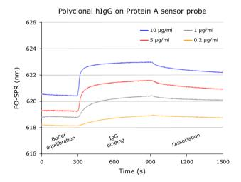
Figure 3. A sensorgram illustrating the responses generated by 4 different concentrations of hlgG ( $\mu$ g/ml) on a Protein A sensor surface including buffer equilibration (baseline) and optional extended association and dissociation steps.
