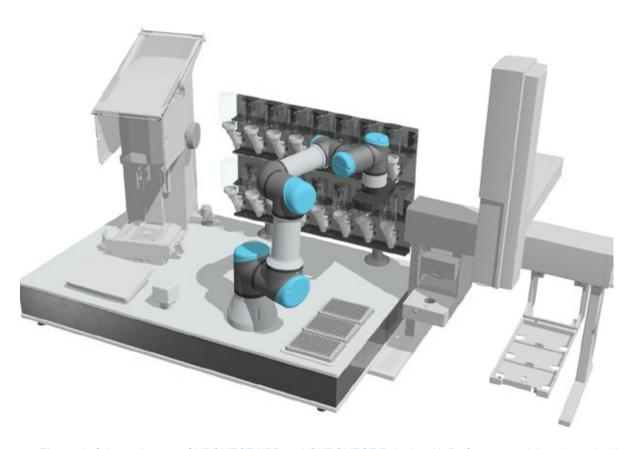
Figure 3: Schematic setup CHRONECT XPR and CHRONECT Robotic with DeCapper module and tray holders.
