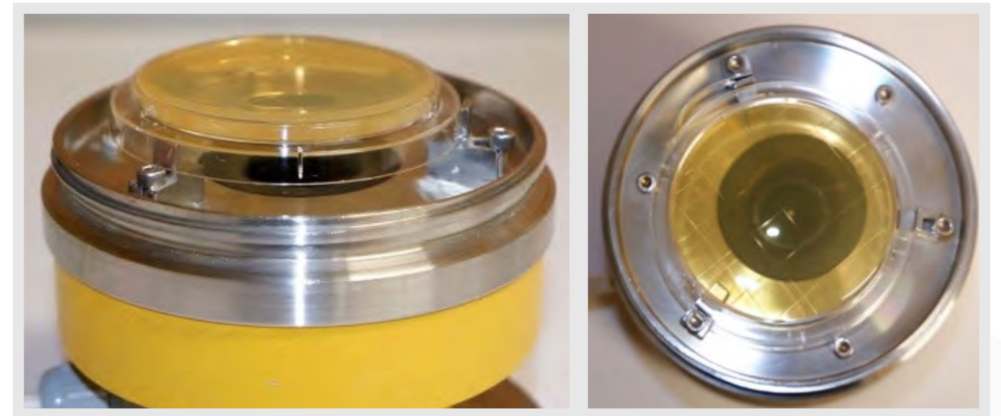
Figure 6 & 7 - Supplier misalignment in samplers
