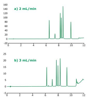
**Figure 1**. Oligo Standard 6 separation on Chromolith<sup>®</sup> RP-18e, 100 x 4.6 mm column at flow rates: a) 2 mL/min; b) 3 mL/min with a gradient of 5% B to 15 % B in 10 minutes. Mobile phase A: 50 mM TEAA in water; Mobile phase B: acetonitrile. Note: injection volume for 2 mL/min is 20  $\mu$ L and 5  $\mu$ L for 3 mL/min.
