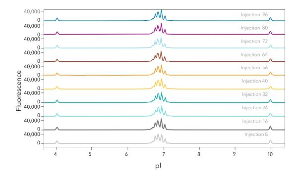
cIEF assay performance over 100 injections with peak area CVs consistently less than 4%. 0.25 mg/mL mAb prepared with 4% 3-10 Pharmalyte, 10 mM arginine and iminodiacteic acid (IDA), pl markers 4.05 and 9.99.
