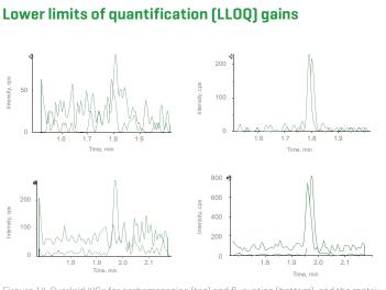
Firgure 14. Overlaid XICs for carbamazepine (top) and fluoxetine (bottom), and the matrix blank (left) and LLOQs (right) for Zeno trap enabled (1x injection volume) and disabled (10x injection volume).
