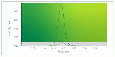
Figure 15. Targeted metabolite quantification. Significant sensitivity gains in MS/MS. Comparison of extraction ion chromatograms (XICs) for cAMP fragments obtained from MS/MS collected with Zeno trap on vs. Zeno trap off. Signal/noise ratio improved ~12.5 fold when using the Zeno trap.
