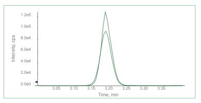
Figure 16. Better sensitivity in MS/MS with 10x less sample. Comparison of extraction ion chromatograms for cAMP fragments obtained from MS/MS collected with Zeno trap on [0.2  $\mu$ L injection] vs. Zeno trap off [2  $\mu$ L injection].
