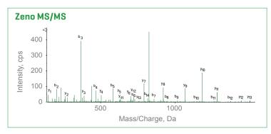
Figure 5. Impact of using Zeno trap for IDA. The Zeno CID MS/MS is shown for the precursor in Figure 6. For a low abundant precursor a high quality MS/MS for identification is acquired with near complete sequence coverage and excellent signal to noise.
