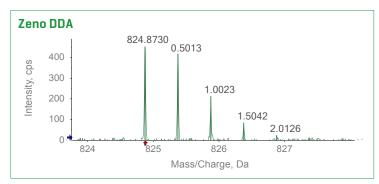
Figure 4. Impact of using Zeno trap for IDA. The TOF MS is shown for a peptide at 25 ng sample load which was triggered for the Zeno MS/MS. The isotopic fidelity is shown up to the M+4 isotope.
