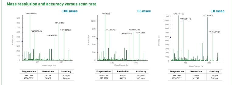
Figure 2. Resolution and accuracy versus scan speed for the ZenoTOF 7600 system. MS/MS resolution and mass accuracy is maintained even at fast scan speeds.
