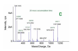
Figure 9. [A] Example peptide from the PQ500 kit with the Zeno trap deactivated; [B] example peptide from the PQ500 kit with the Zeno trap activated for Zeno CID MRM<sup>HR</sup>; [C] Zeno MS/MS spectrum showing mass resolution across the spectrum with a 20 ms accumulation time.
