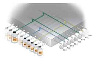
This proprietary matrix valve block system was specifically designed to minimize dead volumes, eliminating cross contamination and delivering peptides with high crude purity.
