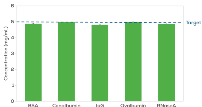
Figure 4: Protein concentration by A280 of 5 mg/mL BSA, conalbumin, IgG, ovalbumin, and RNaseA in PBS. Error bars represent standard deviation.
